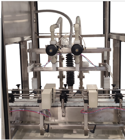
2 corrosive filling nozzles
